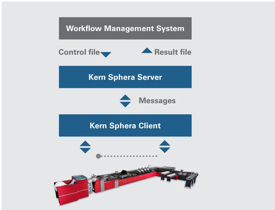
**Sphera DocumentControl directly controls the mail piece processing based on the reading at the entrance of the inserting system.**
